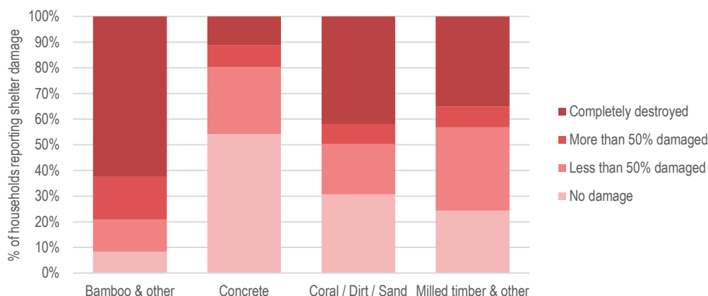
Figure 20: Floor damage, by material
